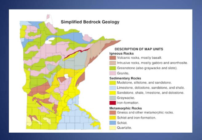
Understand the bedrock geology of the state to identify crushed stone sources
